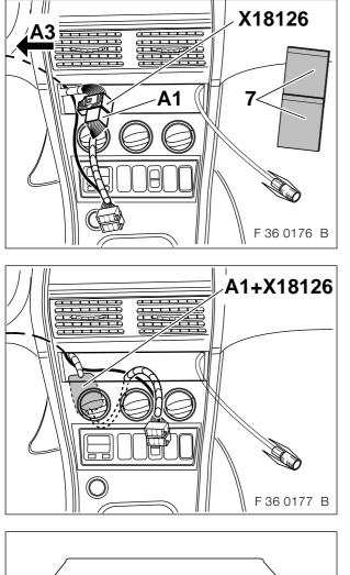
Connect branch **A1**, black 17-pin plug casing on the adapter cable **A** to the black 17-pin socket casing **X18126** on the audio wiring harness. Affix a rattle guard (7) to the second rattle guard (7) and then affix them over the plug connection **A1+X18126**. Lay branch **A3**, exposed cable end, blue/yellow cable on the adapter cable **A**, along the standard wiring harness to the **A** pillar on the left-hand side and secure it with cable ties.
