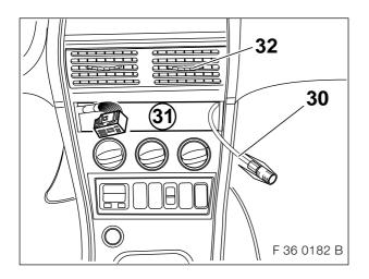
Lay the connection cable (30) for the GPS aerial to the installation site of the radio (31) and tie it back.
