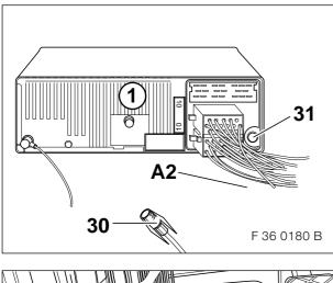
Connect the coaxial plug (30) for the GPS aerial into the coaxial socket casing (31) in the navigation radio (1).
