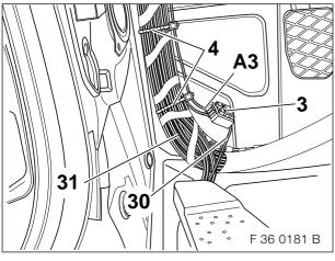
Connect branch **A3**, exposed cable end, **blue/yellow** cable on the adapter cable to the cable for the reversing light (30), **blue/yellow** cable on the main wiring harness (31) with an insulation-piercing connector (3) and secure it with cable ties (4).
