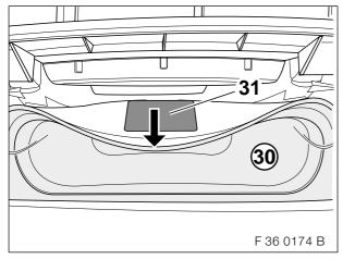
The figure shows the installation space behind the centre fresh air grille. Carefully press the air duct (30) for the centre fresh air grille downwards. Clean the area (31).
