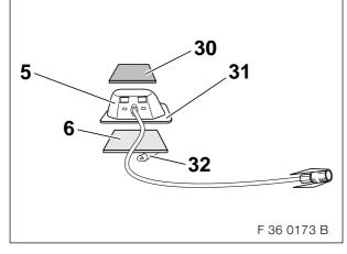
Affix the square (30) of damping strip to the top of the GPS aerial (5) with the retaining plate (31). Affix the adhesive section (6) on to the centre of the underside of the retaining plate (31) and remove the backing foil (32).
