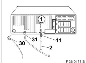
Screw the stud bolt (11) into the navigation radio (1). Screw the radio retaining pin (2) on to the stud
