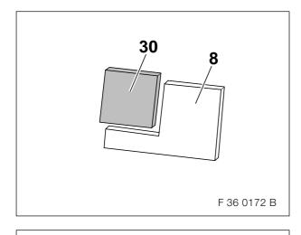
Cut a square (30) measuring 40 x 40 mm out of the damping strip (8).
