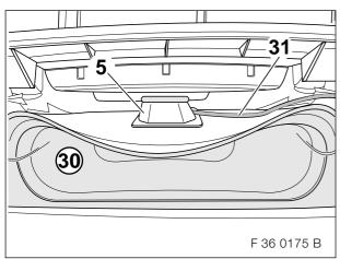
Push the GPS aerial (5) as far to the rear as possible and affix it to the air duct (30) so that the cable outfeed (31) points to the right.
