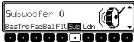
To adjust the subwoofer volume, press the **SOUND** button. Then press the **Sub** multifunction key.
