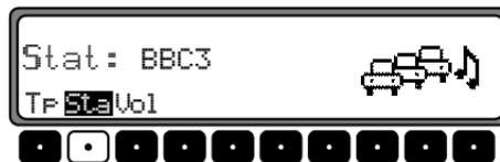
Select the desired TP station by turning the right knob
