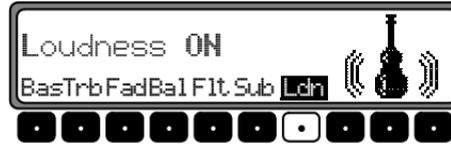
To adjust the loudness, press the **SOUND** button. Then press the **Ldn** multifunction key.
