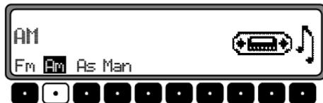
Once you have made your selection, press the **RADIO** button to return to radio mode. The unit will time out and return to radio mode after 8 seconds without pressing a button. The display will show the desired data (frequency, time, etc.) upon returning to radio mode.
