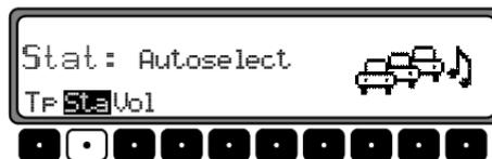
Select Autoselect with the right knob
