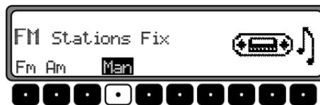
Press the **Man** multifunction key twice. Next, turn the right knob ●. Tuning will take place in increments of 200 kHz.
