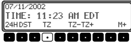
The time zone list will be displayed. Select the desired time zone from the list by turning the right knob
