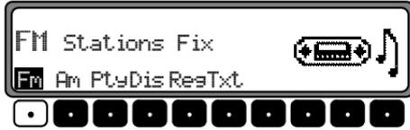
Select the operational level for FM by repeatedly pressing the **Fm** multifunction key. Selection can be made between Stations Fix, Stations RDS, DAS Seek Qual., and DAS Seek Name. (See page 76 for descriptions of each of the operational levels.)
