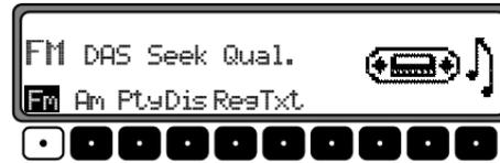
In the FM DAS mode, the receivable stations are displayed above the multifunction keys depending on the settings.
