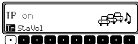
Turn TP off using the TP Menu by repeatedly pressing the **TP** multifunction key until TP off appears.
