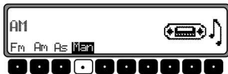
Press the **Man** multifunction key twice. Next, turn the right knob
