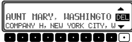
Select the destination to be deleted by turning the right knob
