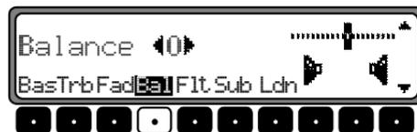
To adjust the balance between speakers, press the **SOUND** button. Then press the **Bal** multifunction key and adjust the balance to the desired level by turning the right knob
