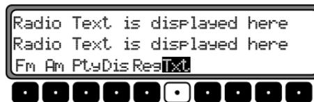
The radio filters information from the data transmitted by the station and displays it in the form of radio text. Radio text cannot be displayed unless the selected station transmits radio text. If the station does not transmit radio text, the display will show “Waiting for Radiotext...” To exit the radio text level, press the **RADIO** button.
