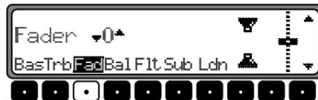
To adjust the fader between speakers, press the **SOUND** button. Then press the **Fad** multifunction key and adjust the fader setting to the desired level by turning the right knob
