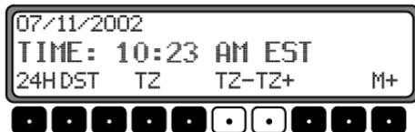
For example, when traveling from Detroit, MI to Chicago, IL you pass from Eastern Time to Central Time. When you pass into the new time zone going west, press the **TZ-** multifunction key. As seen in the example below, the time is decreased by one hour for Chicago time and the display is updated from EST to CST. When returning to Detroit, simply press the **TZ+** multifunction key to return to Eastern time.
