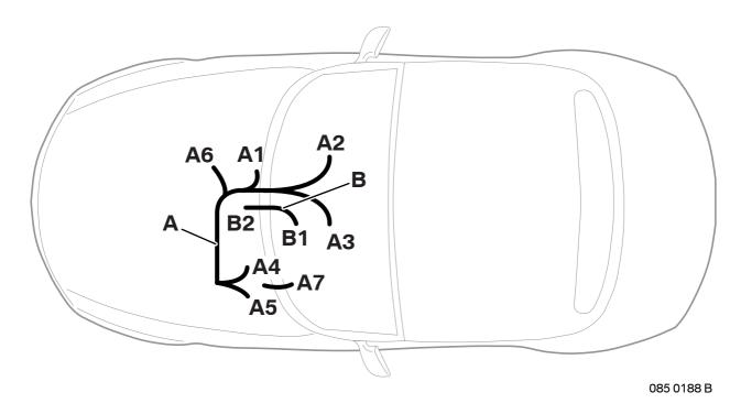
All wiring harnesses are to be installed as shown in the illustration and secured with cable ties. Tie back excess length.
